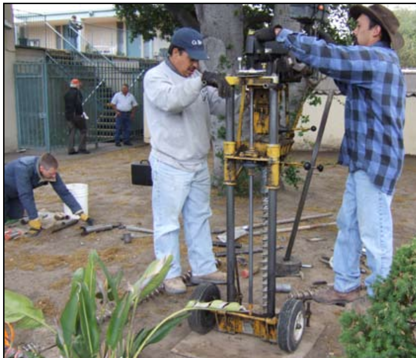
In March, geotechnical studies (core samples of soil) were conducted in connection with proposed CCSM Memorial Garden.
